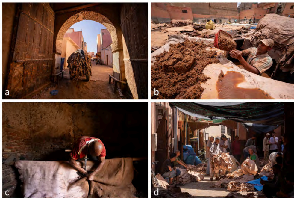
Fig. 15: Marrakech, a: Loaded cart carrying raw skins from sūq a-jeld to the tannery b: Tanner adding more cork oak bark to vat after “breathing” the skins c: Tanner using the sedriya on a cow skin d: dellāl showing finished goat leather to buyers at sūq lbṭāna (Photos: Abdellah Azizi).
